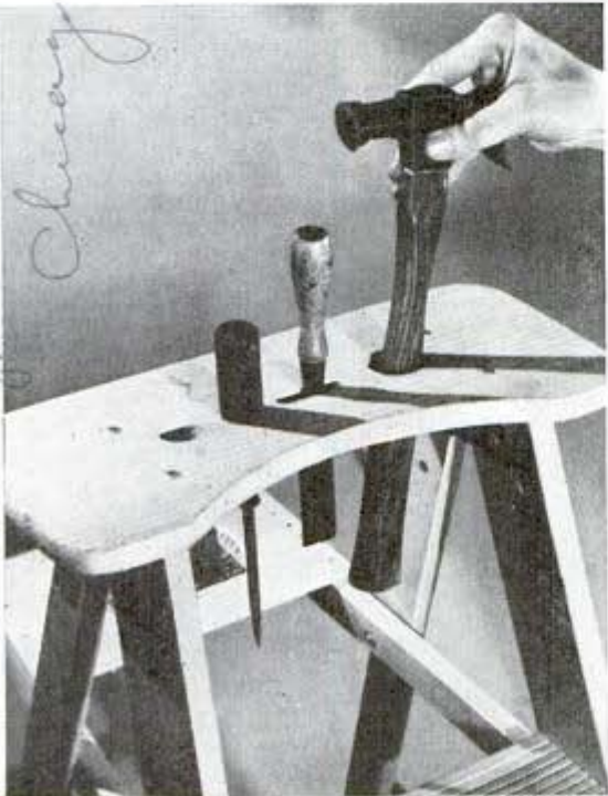
Slots in top of ladder fit the various tools, which are kept from falling and are always in easy reach
